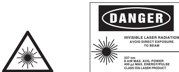
Figure 2-1: These CE and CDRH standard safety warning labels would be appropriate for use as entry warning signs (EN 60825-1, ANSI 4.3.10.1).
